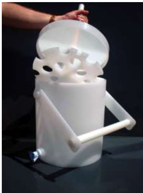
Figure 3 – Suspended sediment and water quality churn splitter used to accurately subsample composited suspended sediment samples
