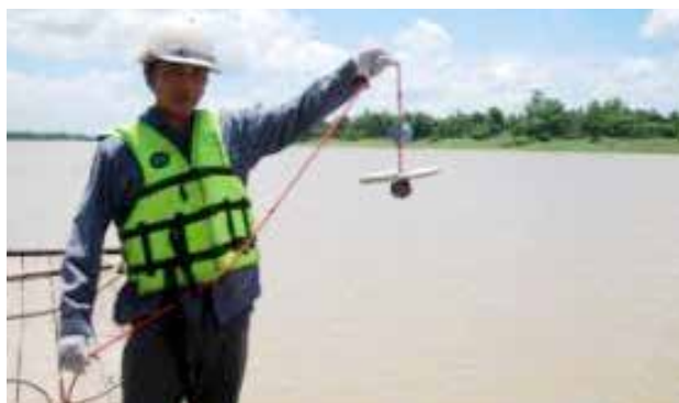
Transparency measuring by Secchi Disc
