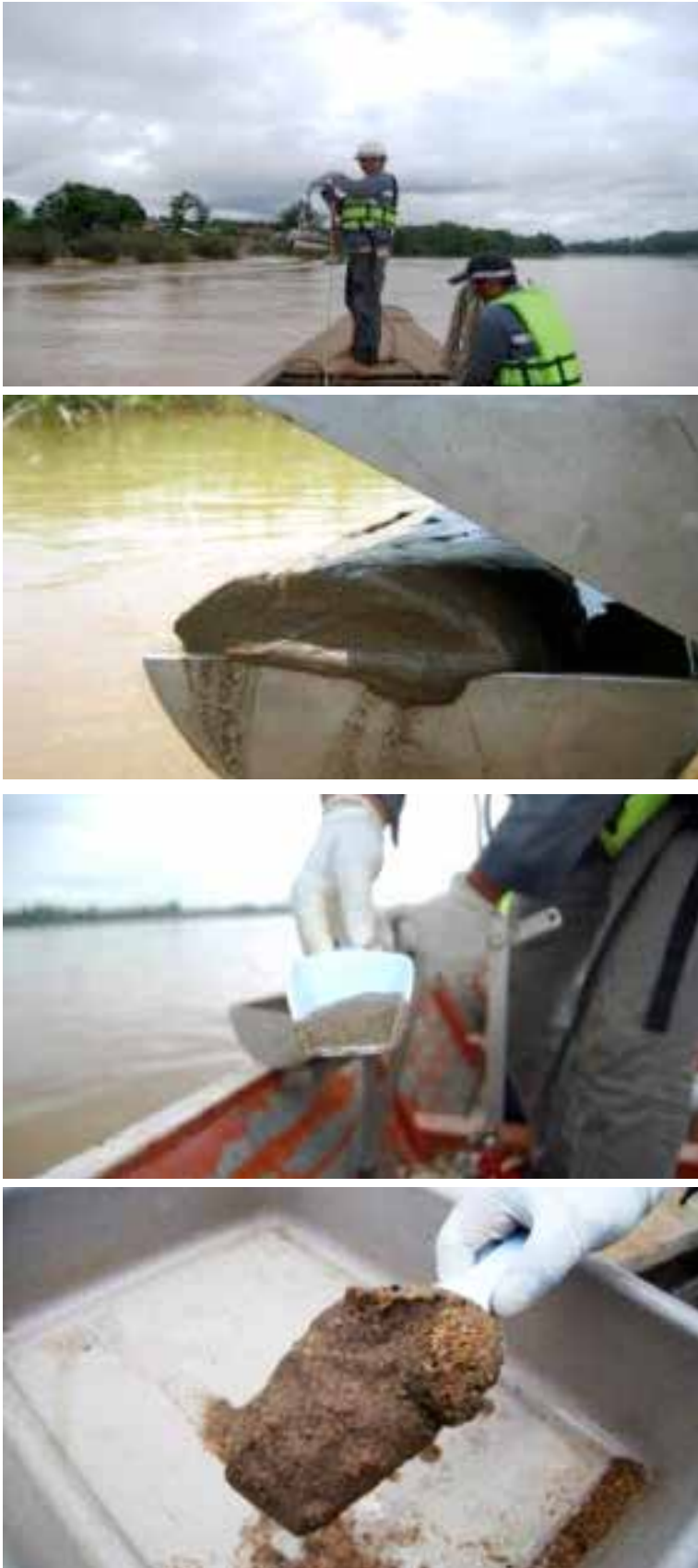
Figure 2-3: Bottom sediment sampling
