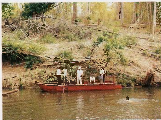
Measuring the river flow near the Ya-Soup dam site
