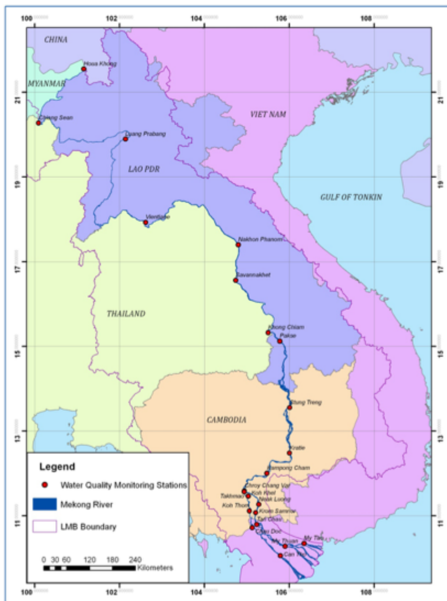
Figure 2.1: Water quality monitoring stations of the MRC WQMN in the Mekong and Bassac Rivers
